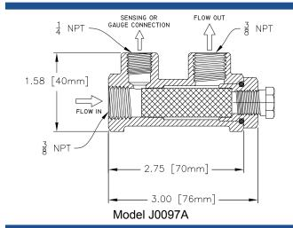
Standard Materials: Body: Stainless Steel 316 Screen Retainer: Stainless Steel 316 Screen (40 Mesh): Stainless Steel 316 Screen Retainer Seal: Buna Blow Down Plug: Stainless Steel 316
