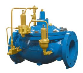
When the valve is modulating to sustain upstream pressure above the minimum 81-RP pilot set-point, the downstream 160 PR pilot may try to open the valve to maintain its set-point, but upstream has priority and downstream pressures will fall below expectations. In typical applications, the standard port model 206-PR-R is often the best selection.
