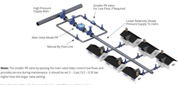
Singer single rolling diaphragm technology 6" / 150 mm and larger have extremely precise control, even at low flows, making smaller by-pass valves unnecessary except for possible bypass during maintenance.
