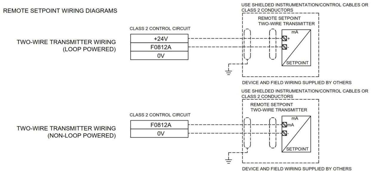
Note: The control panel monitors the health of the control signals and its loss is indicated by an alarm. An alarm relay can be set to remotely monitor the status of the process variable and remote setpoint.
