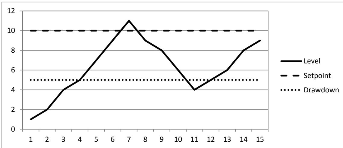
Figure 1: Example of Level Modulation with On/Off Control
